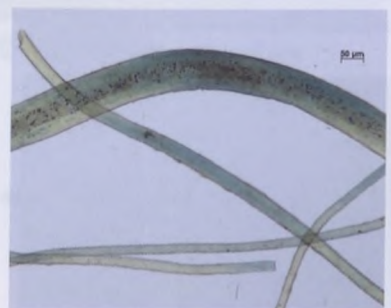
Fibres with indigotin aggregates, light micr. (RHK)
