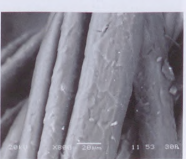
Fibre with degraded scales, SEM 800x (IJ)
