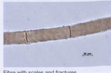
Fibre with scales and fractures, light micro. 400x (RHK)
