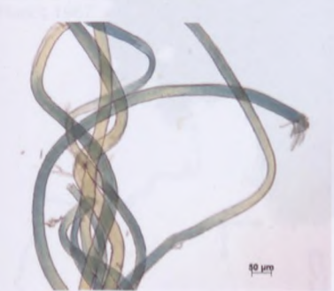
Fibres with indigotin aggregates, light micr. (RHK)
