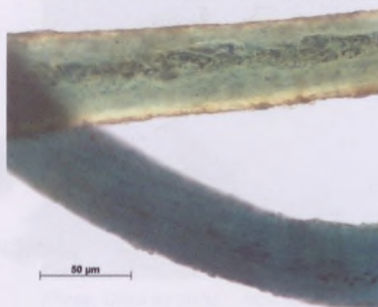
Fibres with indigotin aggregates, light micr. 400x (RHK)
