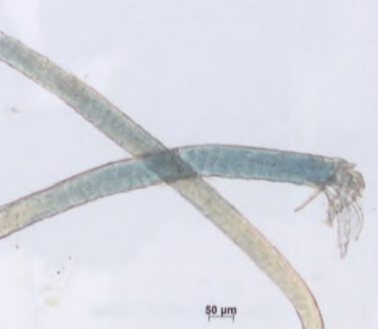
Fibres with indigotin aggregates, light micr. (RHK)
