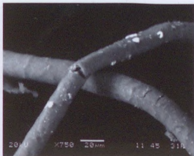
Fibre with fracture, SEM 750x (IJ)
