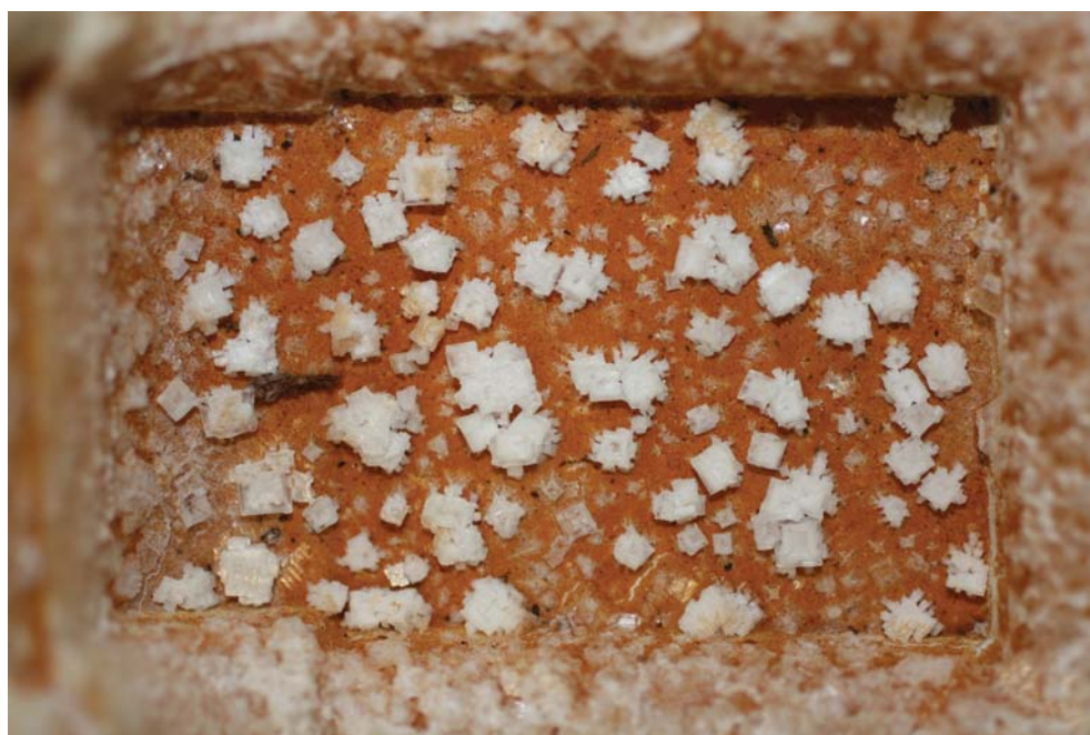
Fig. 2. a: crystallization of salts in the wood fibres; b: in the desalination solution.
